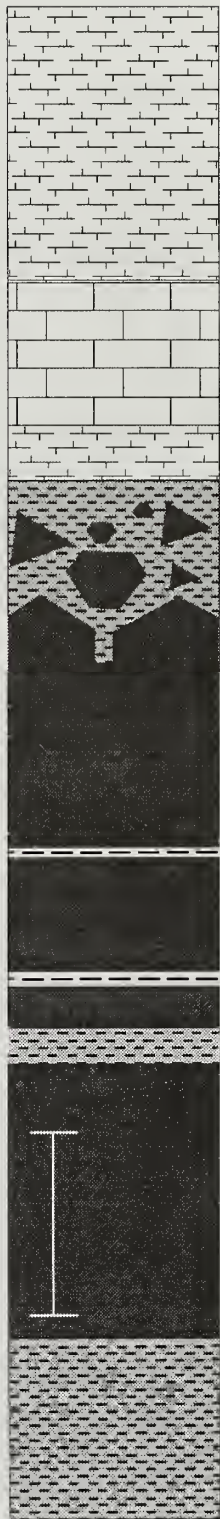
Figure 3-6. Stratigraphic column of strata exposed at Stop 2. The formally named units at this exposure are the Herrin Coal and the Brereton Limestone. A boundary between transgressive-regressive units is at the base of the calcareous shale between the coal and the limestone. The Covell Conglomerate is described at Stop 4. See Figure 3-9 for explanation of lithological symbols used on the stratigraphic column. Vertical scale bar equals one foot.
